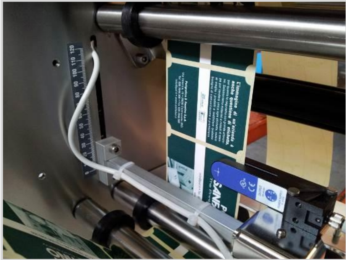
Photo 9.7 Adjustment of the label photocell
