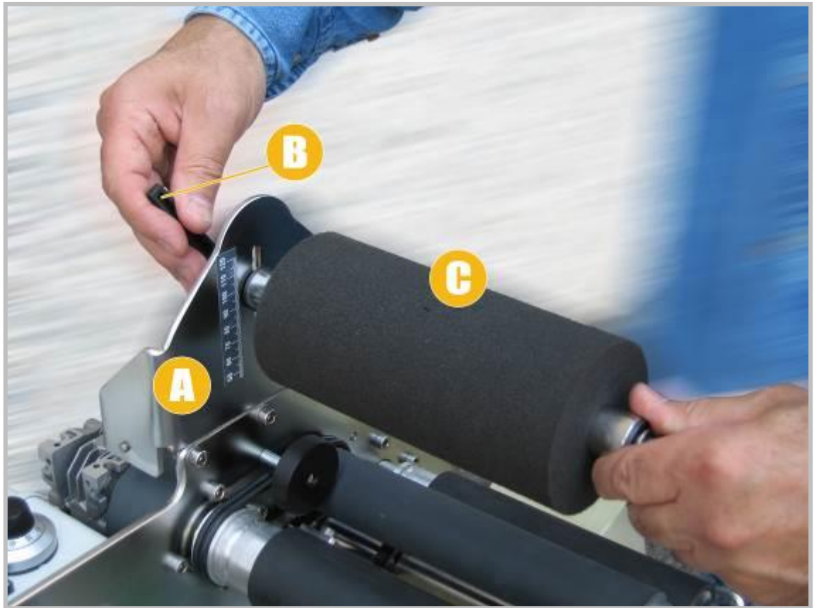
Photo 9.4 Adjustment of the container's diameter
