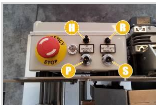
Photo 9.12 Control panel with selector for square bottles.
